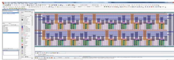
Figure 11 L-Edit IC layout
